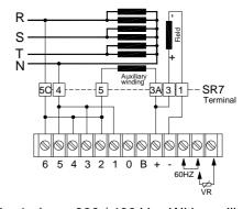
Figure 17 1 phase 380 / 480 Vac With auxiliary winding
