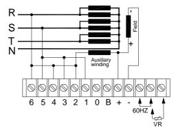
Figure 7 1 phase 220 Vac With auxiliary winding
