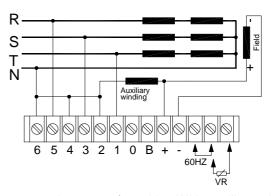
Figure 11 3 phase 380 / 480 Vac With auxiliary winding
