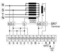
Figure 15 1 phase 220 Vac With auxiliary winding
