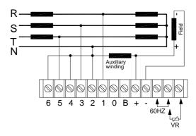
Figure 13 3 phase > 480 Vac With auxiliary winding
