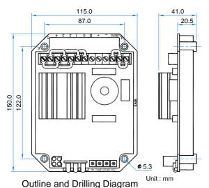
The AVR is equipped with adjustable under frequency protection and over voltage protection to prevent generator from overloading and over excitation.
