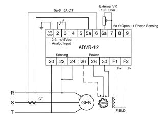
Figure 4 Single Phase Sensing PMG or Auxiliary Winding
