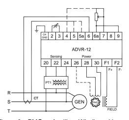
Figure 6 PMG or Auxiliary Winding with power transformer
