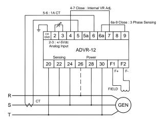
Figure 3 Three Phase Sensing SHUNT
